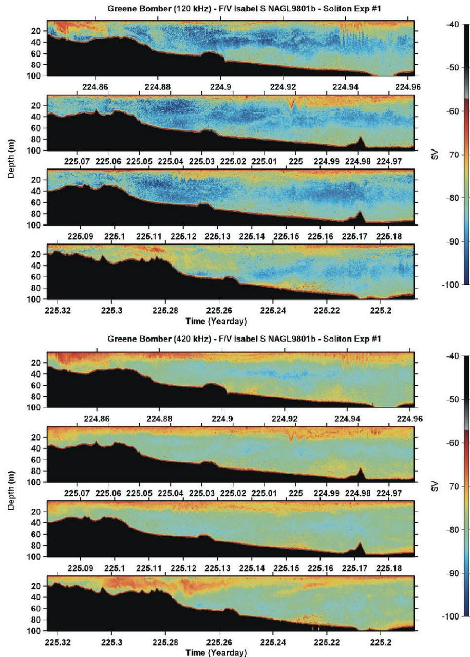
Figure 6. The first acoustic survey between Scituate, Massachusetts and Stellwagen Bank. Data from the 120kHz echosounder are in the top four panels while the 420 kHz data are displayed in the bottom four panels. The survey began in the top panel with the ship steaming east towards Stellwagen Bank (left to right).
