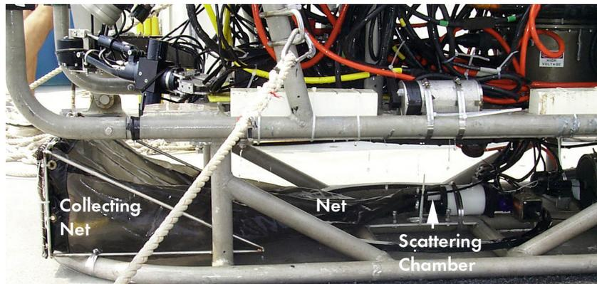
Figure 3. The Acoustic Properties of Plankton (APOP) collection and in situ measurement components mounted beneath the Kraken ROV.
