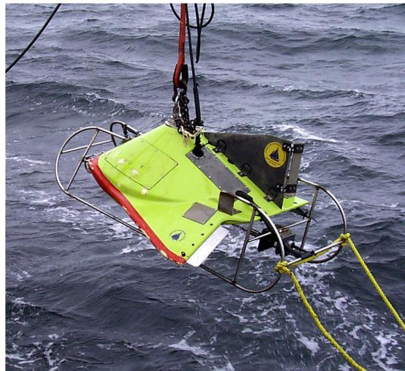
Figure 4. The Greene Bomber prior to deployment from the F/V Isabel S. The fluorometer is visible on the front of the vehicle. The echosounders and T/S sensors are mounted beneath it.
