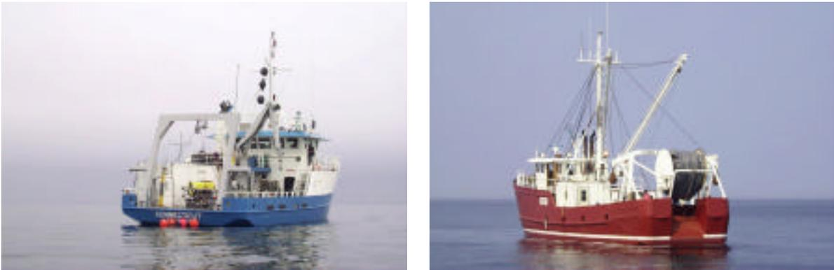
Figure 1. The R/V Connecticut (left) that deployed the Kraken ROV. The F/V Isabel S (right), a commercial dragger, that deployed the Greene Bomber down-looking acoustic system.
