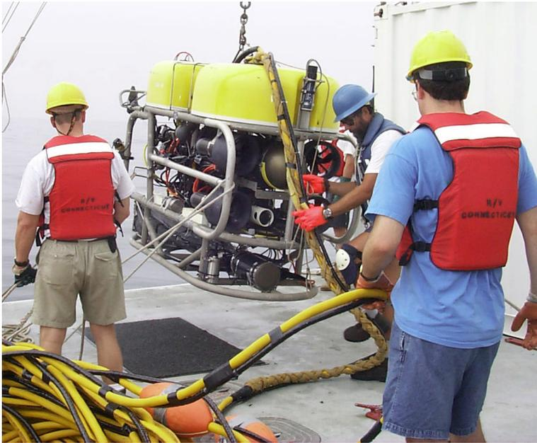
Figure 2. The Kraken ROV (MaxROVER Mk 1) being deployed by Tim Stanton (right), Nick Worobey (center) and Ben Reeder (left) from the R/V Connecticut. The APOP net and one of its pressure cans is visible beneath the vehicle.
