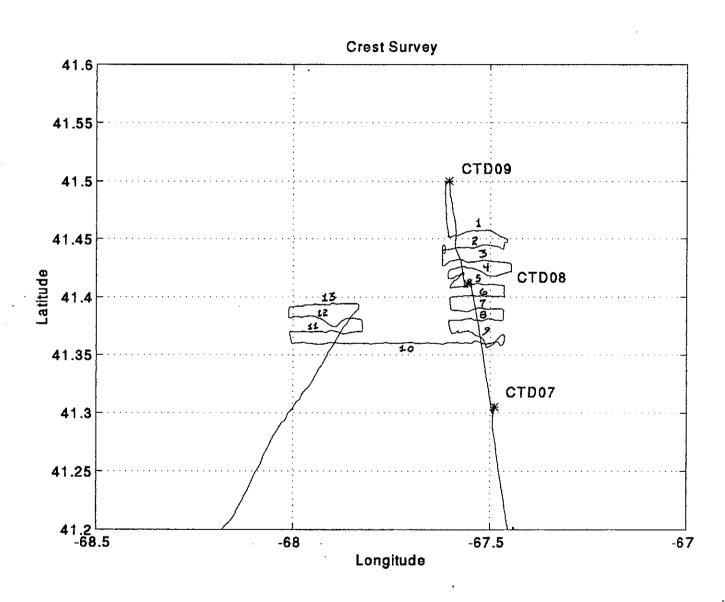
Figure 15. Detail track chart of the Crest PDR Survey indicating the positions of the CTD profiles and the Legs of the Survey at Site A (right) and Site B (left).
