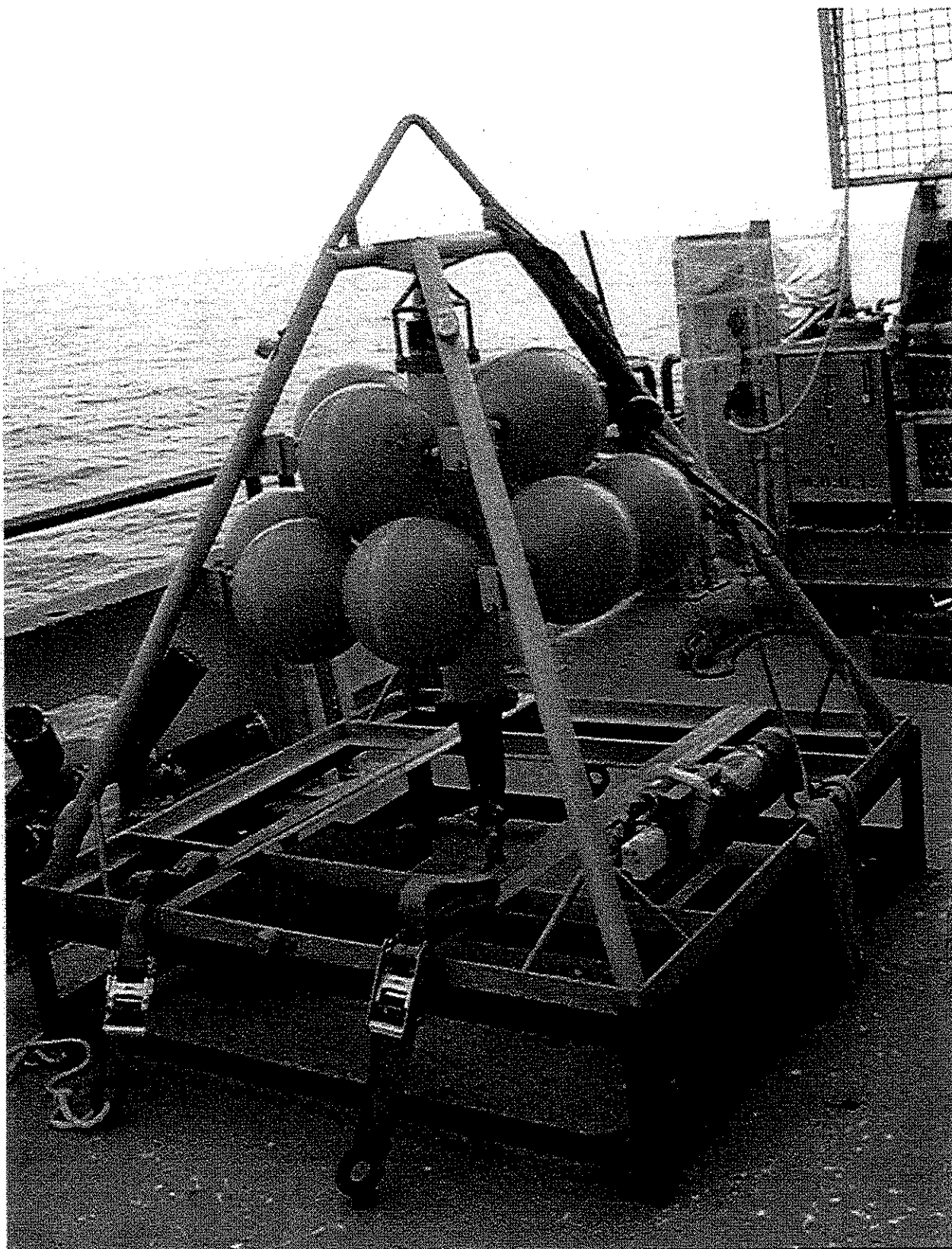
Picture 3. Repaired bottom pressure instrument. The SeaGauge recorder with conductivity on top is seen on the right of the aluminum frame which sits on the steel anchor.
