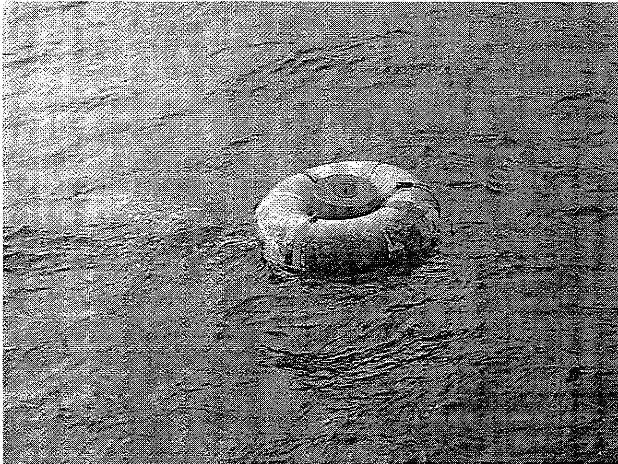
Picture 3. The NSD toroid buoy with center foam plug found floating free of the mooring, upside down on the Northeast Peak of Georges Bank.
