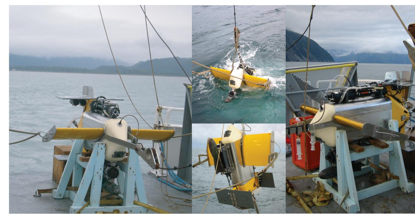
To study these physical regimes of the shelf, we used the SeaSoar--a towed, undulating platform outfitted with various physical, biological and chemical sensors. These sensors collect data about nitrate, fluorescences, chlorophyll, conductivity, temperature, and pressure. The SeaSoar samples 24 data points per second as it moves through the water column, providing (after averaging) one meter vertical resolution while covering two kilometers per cycle horizontally.
