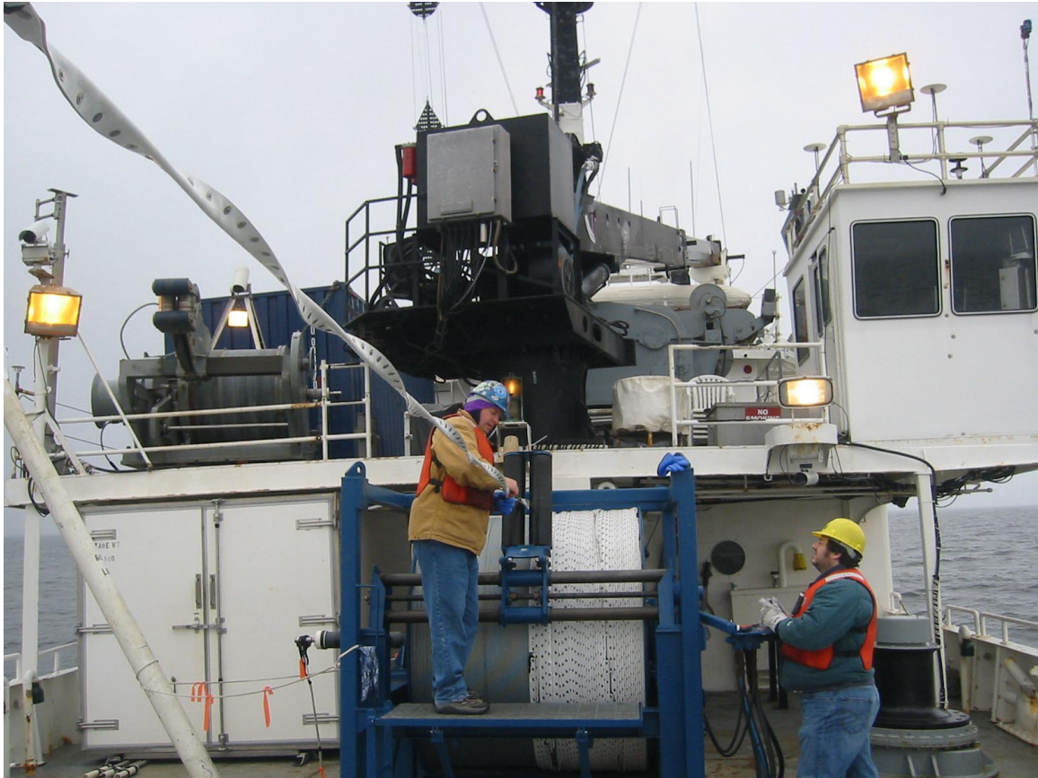
Figure 2. Marc Willis, aided by Toby Martin, removing twisted fairing from the SeaSoar cable. The twisted fairing was causing drag in the water and hindering dive depths.
