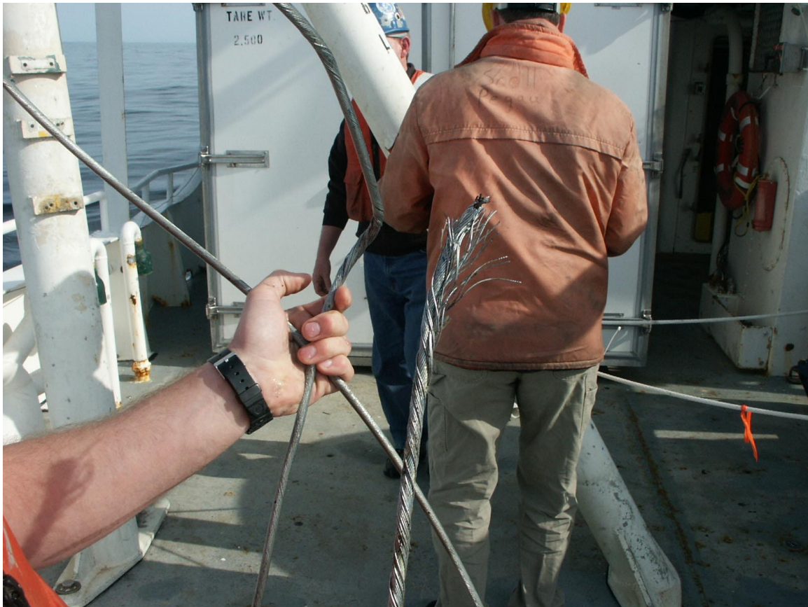
Figure 1. The SeaSoar cable parted at the winch.
