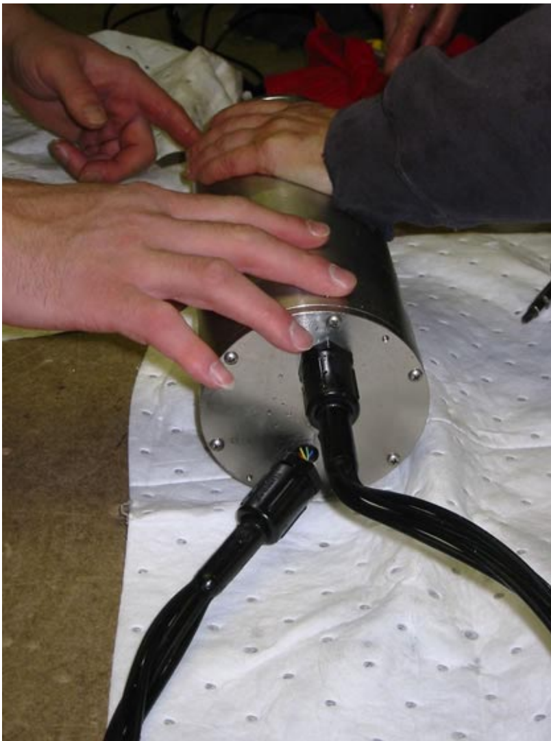
Figure 2. The back of the UFO has a broken connector, which destroys the water-tight seal protecting the power unit.
