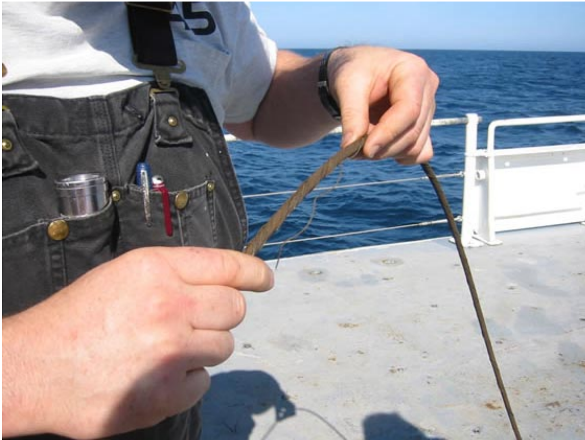
Figure 1. Damaged Tow Cable
