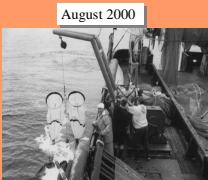
Zooplankton samples were collected prior to each tow using a bongo net that was towed obliquely to 100-m depth.
