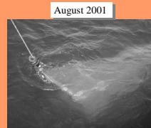
Starting in 2001, zooplankton samples were collected using a 1-m 2 Tucker trawl towed near the surface for 5-minutes.
