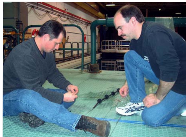
Rigging a model net for testing in a flume tank.
