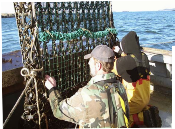
Testing urchin dredge escape panels.
