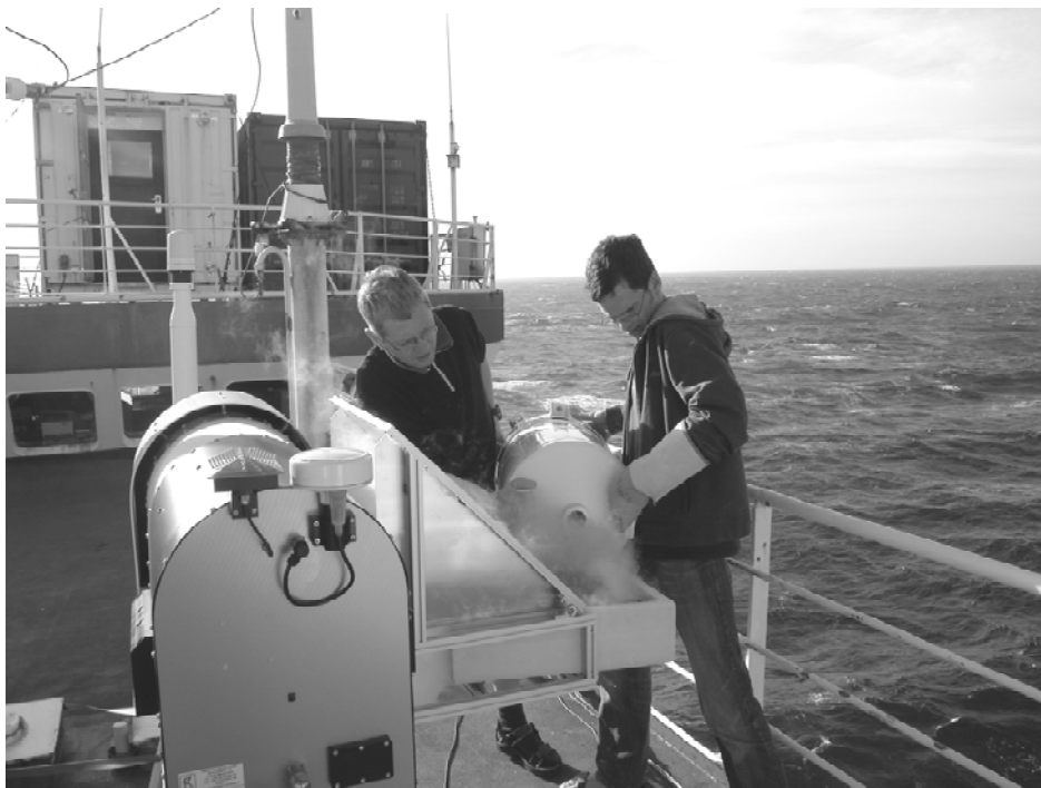
Fig. 1: Calibration of the HATRPO microwave radiometer with liquid nitrogen
