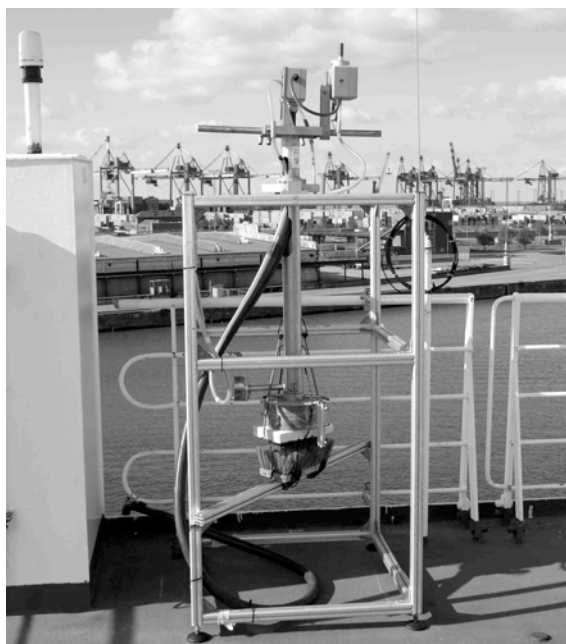
Fig. 4: The on-deck instrumentation of the MAX-DOAS instrument. The telescope unit is mounted on a cardanic system whereby the brush is used for braking the movement influenced by the ship's movement.
