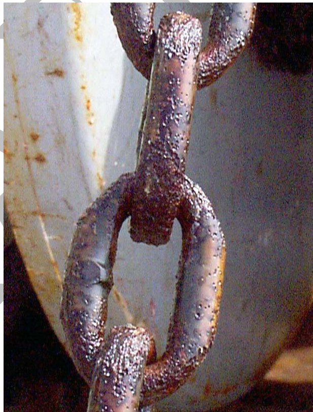
Figure 13. Guard buoy mooring chain. The \frac{3}{4} " chain (upper left) was shiny when recovered. The wear between links is minimal. A recovered anchor (upper right) shows wear due to the motion of the buoy around the anchor. The shackle between the \frac{3}{4} " and \frac{1}{2} " chain (lower left), shows wear on the threads and the nut was only held on by the cotter pin. Finally, the \frac{1}{2} " chain in the water column (lower right) showed pitting and corrosion on the outside of the links, losing up to \frac{1}{2} the material (and strength).
