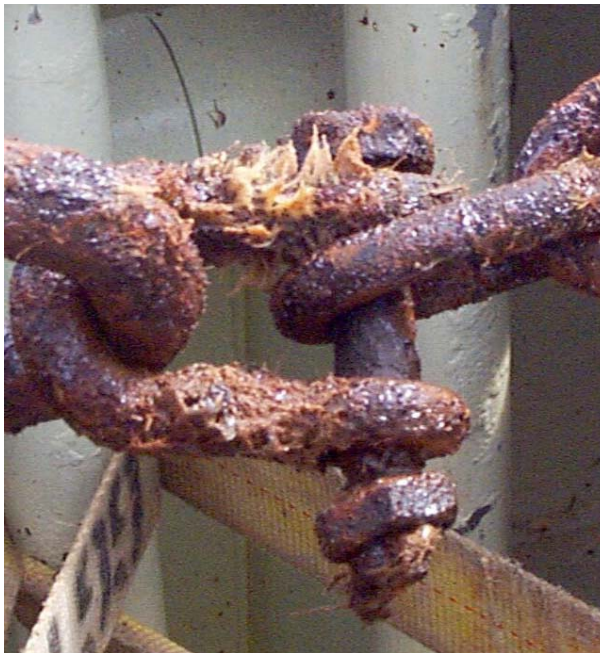
Figure 13. Guard buoy mooring chain. The \frac{3}{4} " chain (upper left) was shiny when recovered. The wear between links is minimal. A recovered anchor (upper right) shows wear due to the motion of the buoy around the anchor. The shackle between the \frac{3}{4} " and \frac{1}{2} " chain (lower left), shows wear on the threads and the nut was only held on by the cotter pin. Finally, the \frac{1}{2} " chain in the water column (lower right) showed pitting and corrosion on the outside of the links, losing up to \frac{1}{2} the material (and strength).
