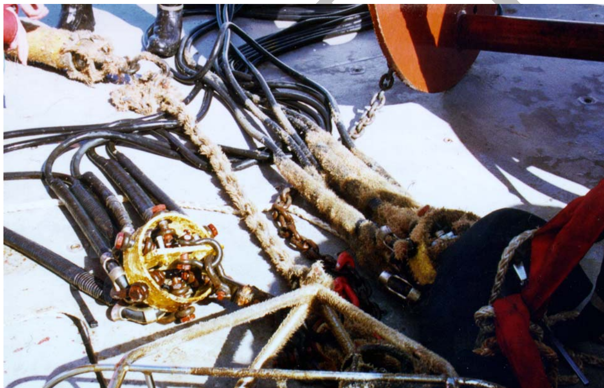
Figure 10. Compliant Elastic Tethers after recovery. The round bridle to which the six 10-m unstretched length elastics are shackled is seen in the left center of the picture. Six 1" diameter tethers are used to give the required stiffness, and the 10-m length provides the compliance to allow the mooring to move with the currents and tides, and still allow the buoy to move up and down with the waves. They provide about 500 lbs downward tension on the buoy.
