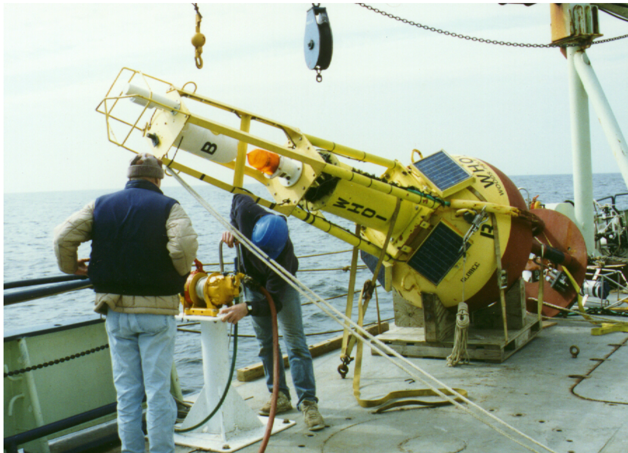
Figure 9 Crest and Northeast Peak buoy on deck of R/V KNORR prior to deployment in April 1997. The PAR sensor can be seen in the buoy tower top, with the Gill radiation shield partially hidden by the GOES/ARGOS antenna. The electronics and batteries are housed in the large cylinder in the base of the tower. Four 10-Watt solar panels provide power for the system. The sensors in the water are identical to the Southern Flank mooring.
