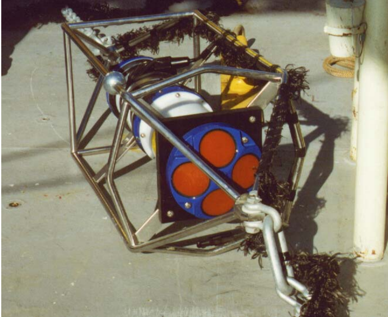
Figure 4. 300-kHz RD Instruments Workhorse ADCP mounted in a downward looking configuration in an in-line frame with auxiliary battery pack. The frame was connected to the buoy with 1 m of chain to decouple the buoy tilting motion from the current observations. The mooring cable (Kevlar strength member with electrical cables and poly anti-strumming hair is the black cable taped to the ADCP frame.
