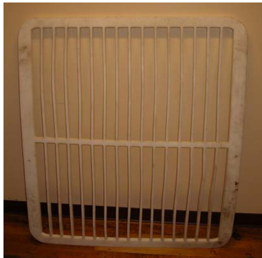
Figure 1: The initial excluder grate, following usage in Phase 1 testing with visible warping in the bars. Image source: /Construction/IMG0239.JPG
