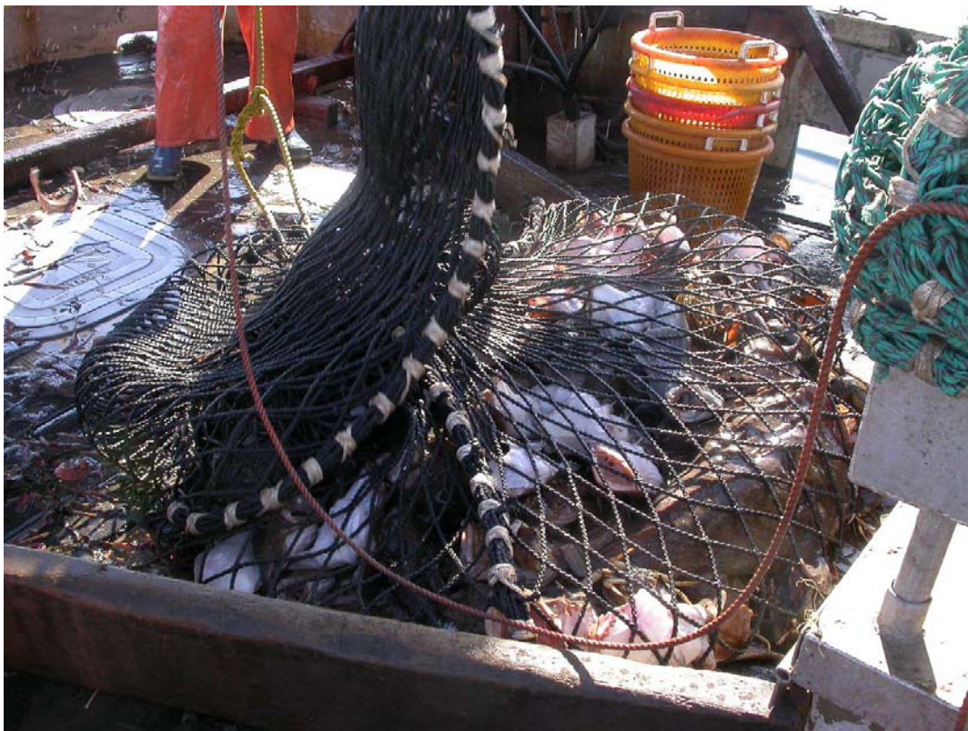
Figure 9. A small catch with knotless twine. The twine handled more easily, and was lighter than its' knotted counterpart.
