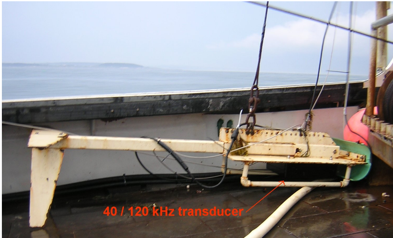
Figure 2. Towed body used to deploy transducers for acoustic surveys.
